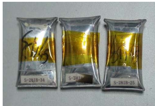
150 °C heating test of HBL
