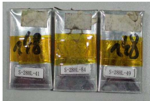
1C/12V over-charge test of HBL
